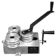
THE 90° LI'L NOTCHER (#1751) is a cutting tool that puts a notch in 1/8" U brass or zinc channel. It allows the came to go around sharp 90° corners without puckering. It saves you having to cut or miter the channel to make corners when using 1/8" channel for borders.
