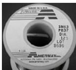
**ONYX 50/50 SOLDER (#MET 5050A)**, while not widely used, is often preferred because of its lower cost. Since it has a higher melting point (melts at 413°F, solidifies at 361°F) it is not recommended for lead came work, but some people prefer to solder the back side of their foiled work with 50/50 first, then solder the front side with 60/40. The difference in melting points helps eliminate solder "run-thru" to the back side.
