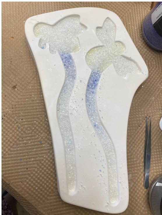
Fill the mold with Clear Medium Grain frit until the mold holds approx. 162 grams of frit. Fire to a full fuse, a suggested full fuse can be found in table 1.
