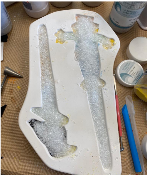
Place Medium Clear frit into the mold cavities until the frit in the mold weighs approx 198 grams. Full fuse the mold using the schedule we suggest in table 1.
