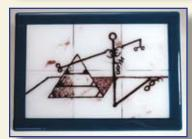
7 - After the piece was fired to 1335 for 10 minutes, the System 96 black frit turned dark and glossy and it texture fused to the surface of the base glass.
