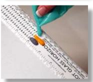
The ramp is easy to make. I just cut a piece of 1 inch thick or is thicker Styrofoam at a 45° angle and tape a smooth surface, such as a plastic ruler or a piece of glass onto the angle slide of the ramp. A ruler is handy, because it gives you accurate measurement on how much your tests sample moves over a given period of time. If you take the time to make a simple ramp and test the consistency of your paste, you will have a much higher success rate.
