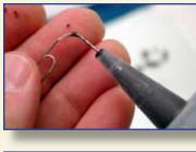
4 - When the paste didn't flow evenly, I cleaned the tip with a piece of wire.
