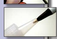
seems to work well. A #4 hole should just accommodate the tip of your average ball point pen. (1.8 mill)
