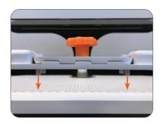
**1. Turn off Grinder.** Center THE SET horizontally across the Lift Grid, in-line with the grinding bit.
