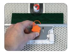
When Adjustable Plate is in desired location, tighten the Adjustment Knob by turning clockwise unit it locks. Remove glass piece.
